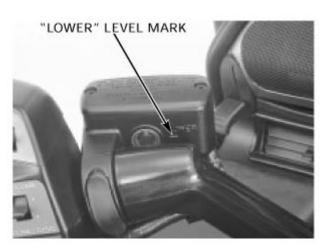
If the level is near the "LOWER" level mark, remove the reservoir cap, set plate and diaphragm, and fill the reservoir with DOT 4 brake fluid from a sealed container to the casting ledge.
