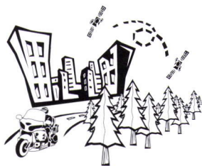
Low GPS satellite position (less than 10 degrees) on the horizon.
